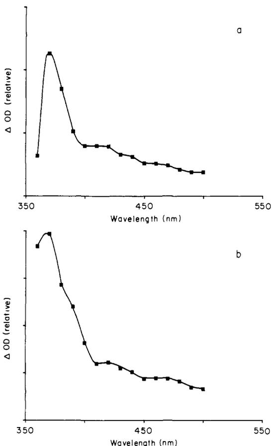
**Figure 10.** Spectra taken directly after photolysis with a 7-ns, 355-nm laser pulse of Ar-saturated  $\text{CH}_3\text{CN}$  solutions of 4t-Urd (a) and DMTU (b) that contained saturated ( $<0.1$  M) TEA. Near-complete excited-state quenching and electron transfer are both observed. Absorption at 370 nm is due to the thiouracil anion radicals, while the weak, broad visible absorption is assigned to  $\text{TEA}^+$ .
