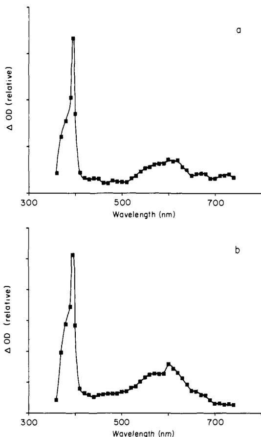
Figure 8. Spectra taken directly after photolysis with a 7-ns, 355-nm laser pulse of Ar-saturated  $\text{CH}_3\text{CN}$  solutions of 4t-Urd (a) and DMTU (b) that contained 0.05 M  $\text{MV}(\text{BF}_4)_2$ . Near-complete excited-state quenching and electron transfer are both observed. The spectra readily show the absorption of  $\text{MV}^+$  ( $\lambda = 395$  and  $600$  nm) and suggest the appearance of weak absorption from 400 to 500 nm due to the thiouracil cation radicals.
