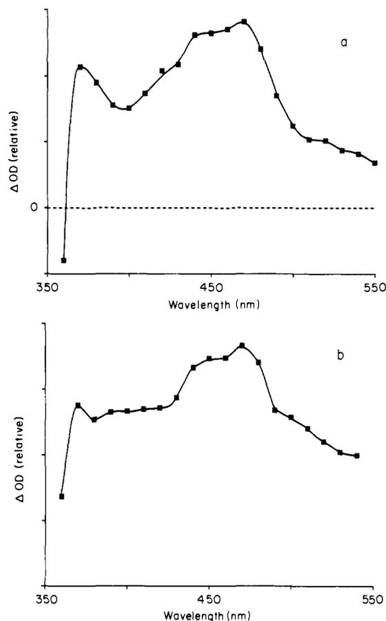
Figure 9. Spectra taken directly after photolysis with a 7-ns, 355-nm laser pulse of Ar-saturated  $\text{CH}_3\text{CN}$  solutions of 4t-Urd (a) and DMTU (b) that contained 0.3 M DEA. Near-complete excited-state quenching and electron transfer are both observed. Absorption at 470 nm is due to  $\text{DEA}^+$ , while absorption at 370 nm is assigned to the thiouracil anion radicals.
