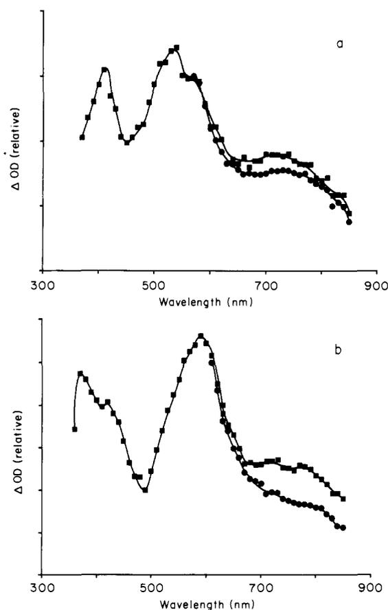
**Figure 4.** Triplet-state absorptions in the visible region of 4t-Urd (a) and DMTU (b) taken directly after photolysis with a 7-ns, 355-nm laser pulse. Spectra of both Ar-saturated (■) and  $\text{N}_2\text{O}$ -saturated (●) water solutions are shown. Note that  $\text{N}_2\text{O}$  decreases the transient absorptions in the red without affecting the blue portions of the spectra.
