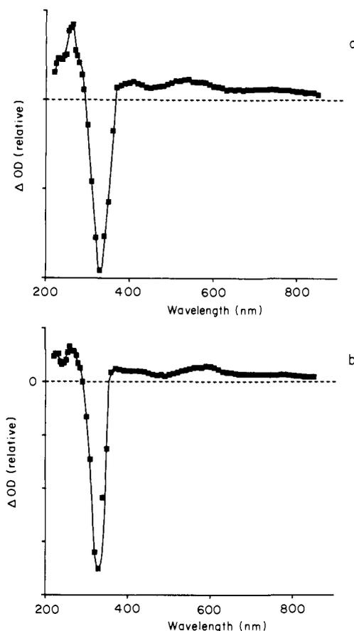
**Figure 3.** Transient absorption spectra of Ar-saturated  $\text{H}_2\text{O}$  solutions of 4t-Urd (a) and DMTU (b) taken directly after photolysis with a 7-ns, 355-nm laser pulse. Note the large signal at 330 nm due to ground-state bleaching relative to the triplet-state absorption in the visible region.
