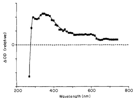
**Figure 2.** Transient absorption spectrum of an Ar-saturated CH<sub>3</sub>CN solution of U at 295 K taken 250–300 ns after photolysis with a 7-ns, 266-nm laser pulse.
